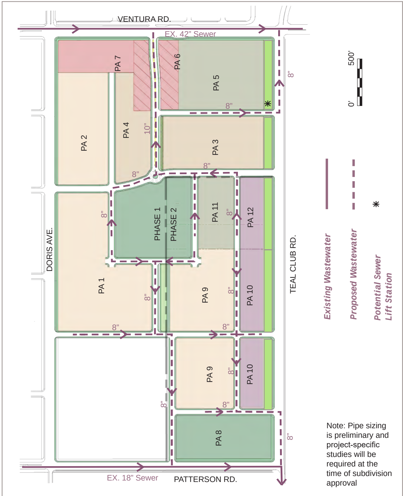
FIGURE 4-16 PROPOSED BUILD-OUT WASTEWATER SYSTEM
