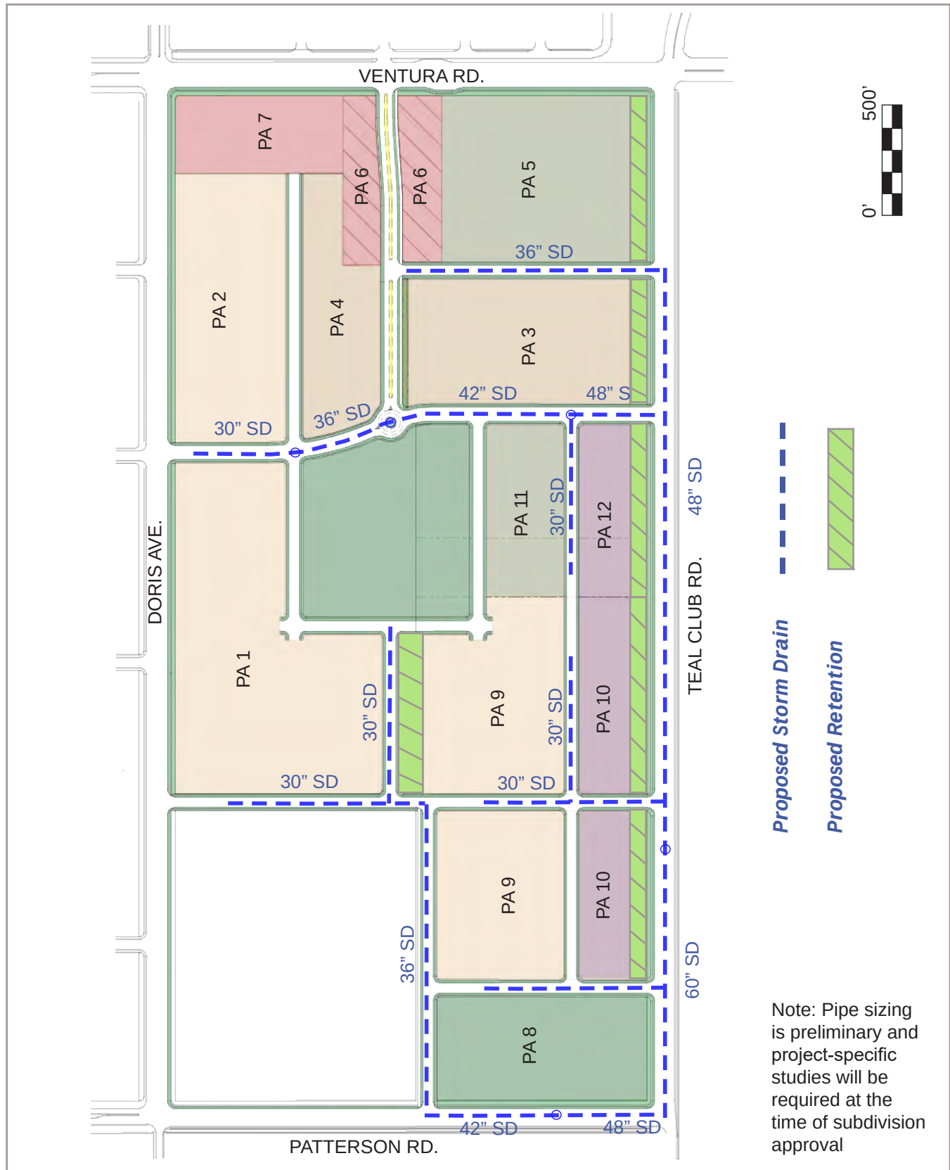
FIGURE 4-18 PROPOSED BUILD-OUT STORMWATER DRAINAGE SYSTEM
