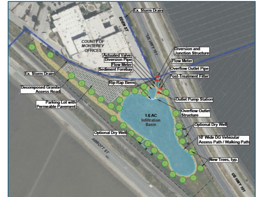
Figure 6: Example infiltration strategy concept in mixed land use location (Salinas, CA)
