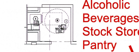
ENLARGED PLAN 1/4" = 1'-0" ICE MACHINE - 3RD FLOOR ONLY
