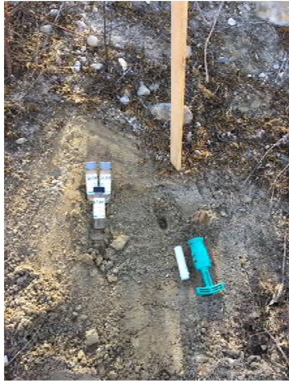
PHOTO #6 DETAIL OF SOIL SAMPLING LOCATION S16-2@0-3". NOTE REMNANT OF ORIGINAL SURVEY STAKE ABOVE T-HANDLE SAMPLER.
