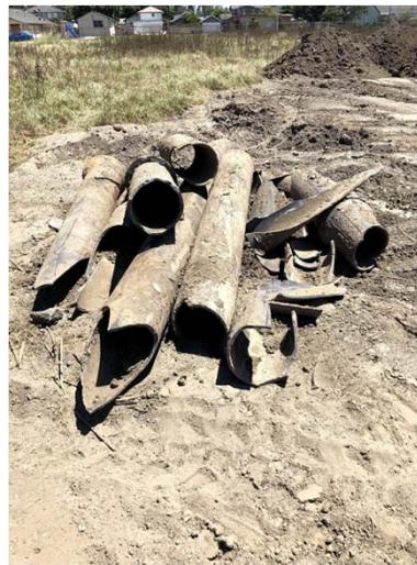
Typical condition of existing 60-year old cast iron pipe
