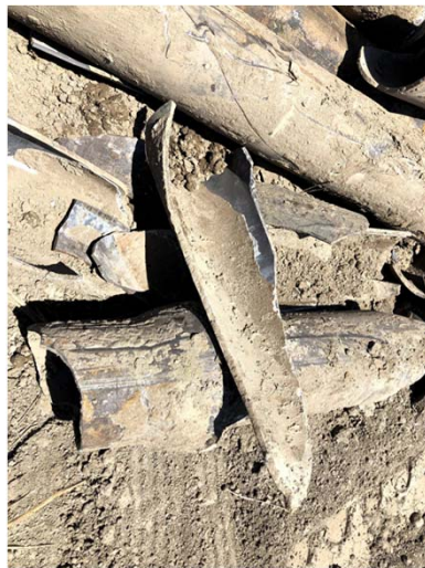
Typical condition of existing 60-year old cast iron pipe
