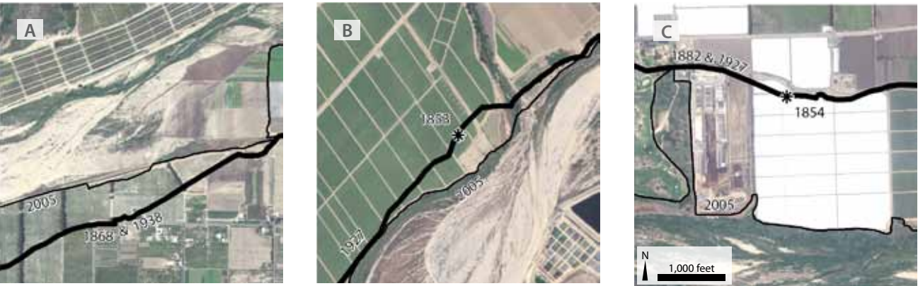
Fig. 3.17. Examples of historical persistence in bank location. In many locations along the river, the position of the outer bank remained quite stable over decades, despite intervening major floods (including the St. Francis Dam break of 1928). This is illustrated here in three reaches: south of the Sespe Creek confluence (left), at South Mountain (middle), and at the Olivas Adobe near the river mouth (right). In each case, early (1854-1882) evidence also confirms the early 20th century (1927-1938) bank position. In each instance, by 2005 bank position has shifted somewhat. (USDA 2009)
