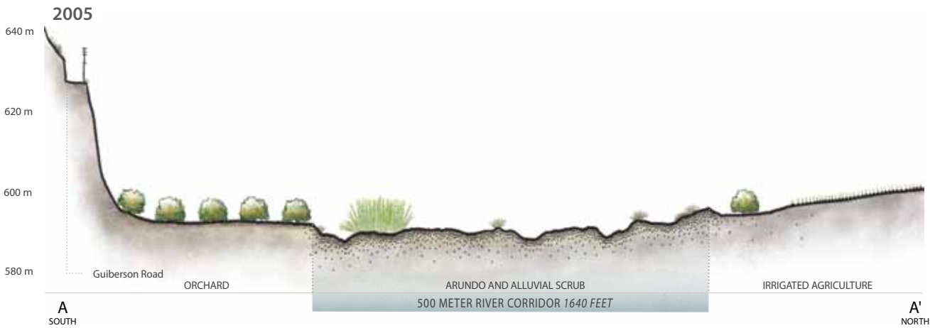
Fig. 3.45. Historical cross-sections at Piru, 1874-2005. This series shows the Santa Clara River west of Piru, between Piru Creek and Hopper Canyon. This intermittent reach was characterized by a broad active channel dominated by sand and scrub vegetation. Similar hydrology and vegetation persist today, though Arundo is now present and the river corridor has narrowed due to agricultural development on the floodplain. Cross-sections are drawn with 5x vertical exaggeration. (Craven 1874f; USDA 1938, courtesy of Ventura County; USDA 2005; Stillwater Sciences and URS Corporation 2007. Cross-sections produced by Jen Natali)
