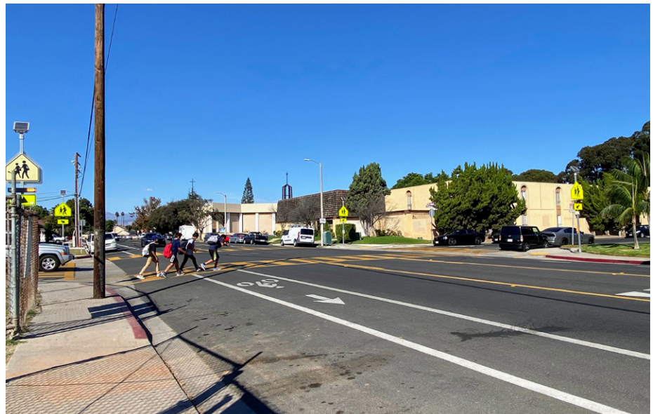
RRFBs alert motorists of a crossing pedestrian with a pedestrian-activated flashing light. Source: City of Oxnard
