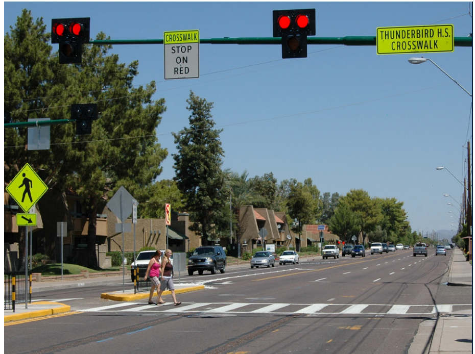
Pedestrian hybrid beacons alert drivers to stop for crossing pedestrians with a series of red and yellow lights. Source: Mike Cynecki, pedbikeimages.
