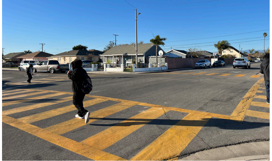
Adding bulbouts at intersections near schools, such as Laurel Street & Gisler Avenue, would shorten pedestrian crossing distances, increasing pedestrian visibility, and potentially provide space for low-level landscaping
