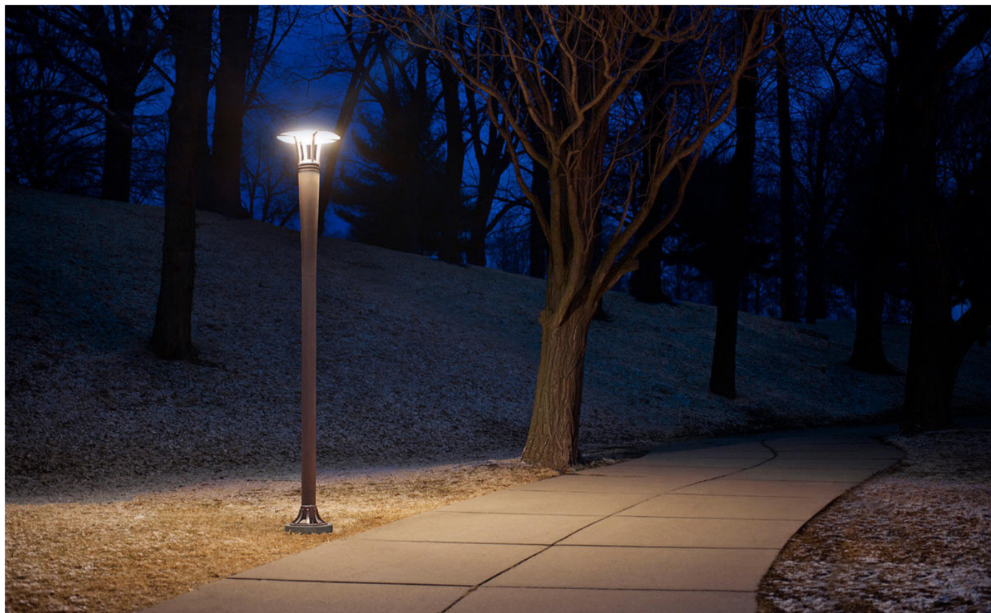
Pedestrian-scale lighting is shorter than roadway lighting to improve visibility for people walking. Source: Forms + Surfaces
