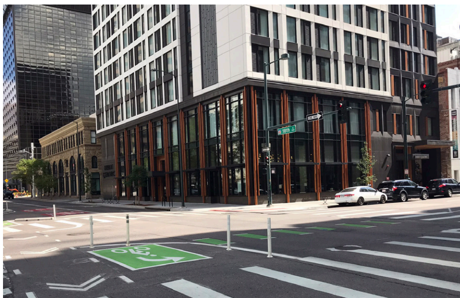
Bike boxes (two stage left turns) offer bicyclists a safe way to make turns at intersections. Source: Laura Sandt, pedbikeimages
