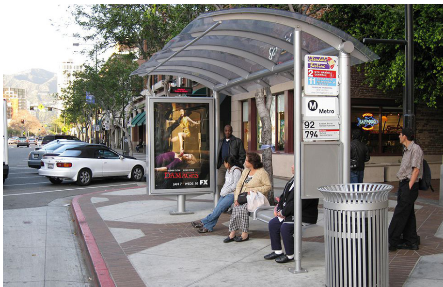
Boarding bulb transit stops align the transit stop with the parking lane to improve passenger loading/unloading efficiency. Source: NACTO.
