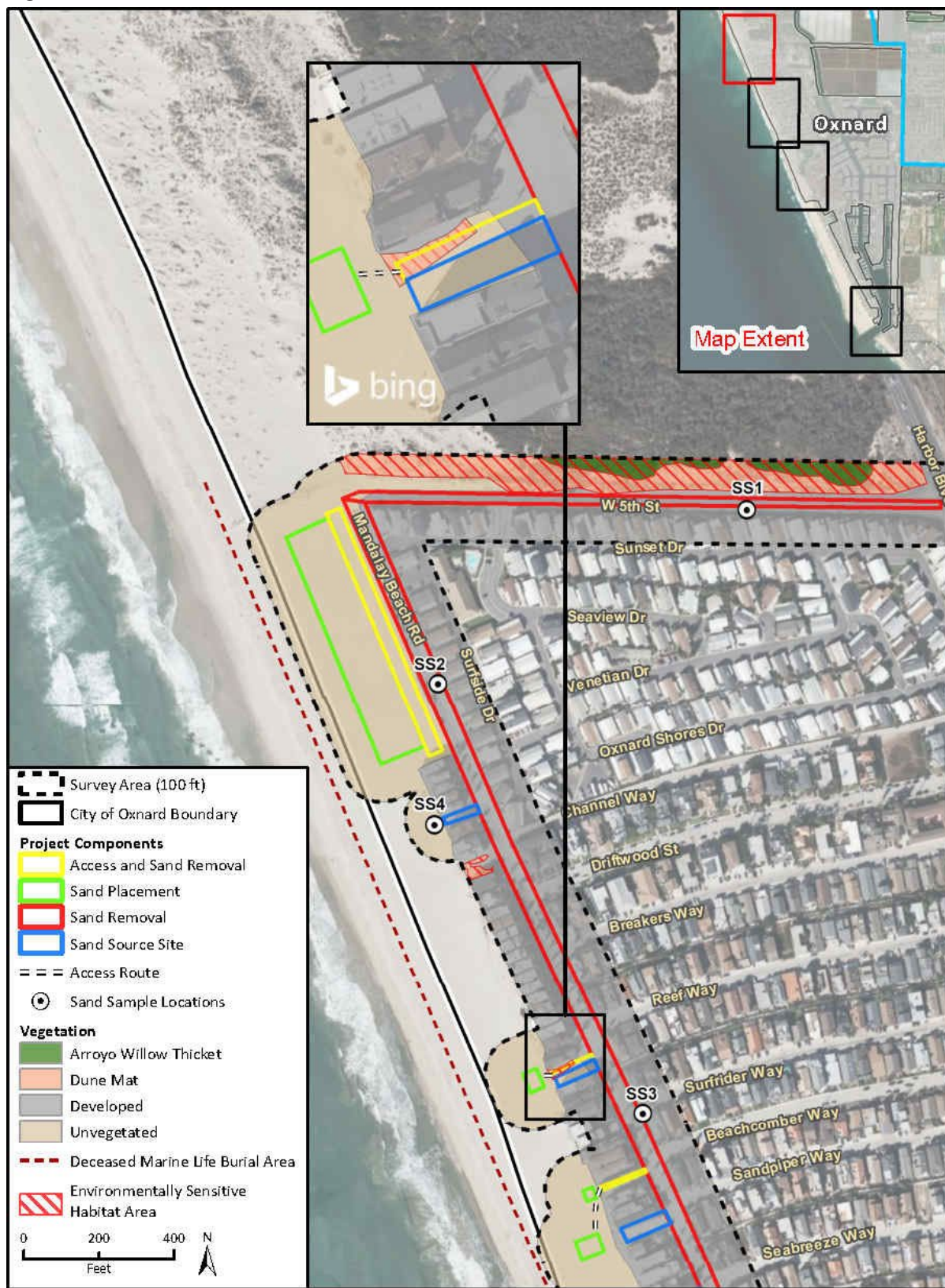
Figure 1 Sand Removal Area 1 - Fifth to Seabreeze
