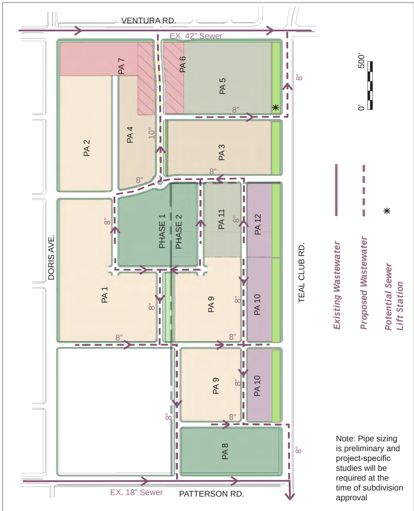
FIGURE 4-16 PROPOSED BUILD-OUT WASTEWATER SYSTEM
