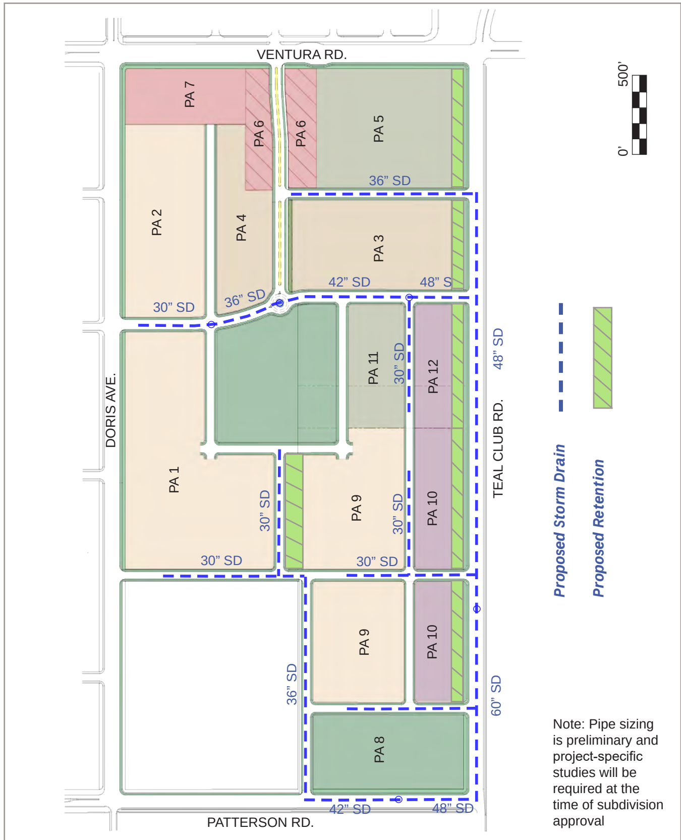
FIGURE 4-18 PROPOSED BUILD-OUT STORMWATER DRAINAGE SYSTEM
